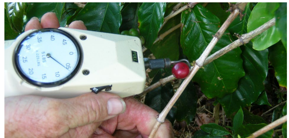
Figure 15.5: Maximum harvesting efficiency is achieved when the ratio of the pull-force required to remove the ripe and unripe cherry is as wide as possible.
