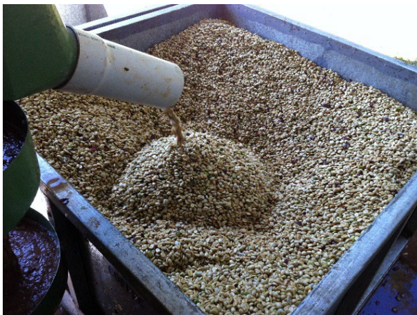
Figure 16.3: Receival – the harvester dumps the cherry crop directly into the receival tank prior to pulping.
