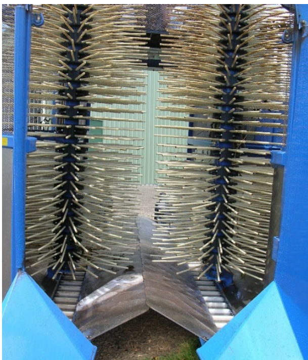
Figure 15.12: The vibration frequency, pressure loading, and amplitude of the harvester's shaker fingers can be adjusted to improve the efficiency of cherry removal.
