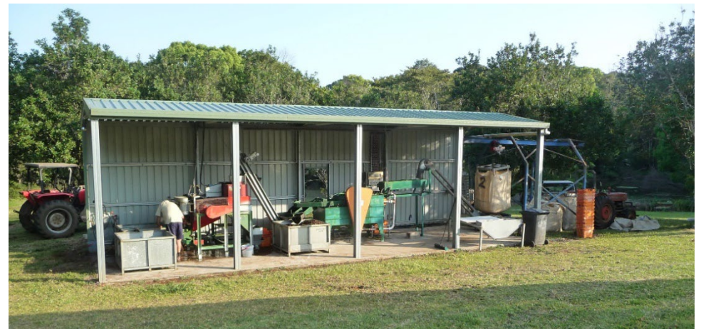
Figure 16.6: Compact in-line processing set-up for smaller operations. Receival is on the right, then passes through leaf shaker, flotation tank, pulper and demucilager.
