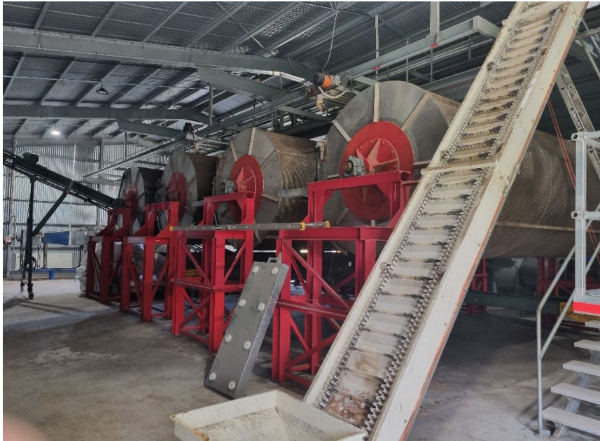
Figure 16.7: Horizontal rotary driers can dry parchment or naturals.
