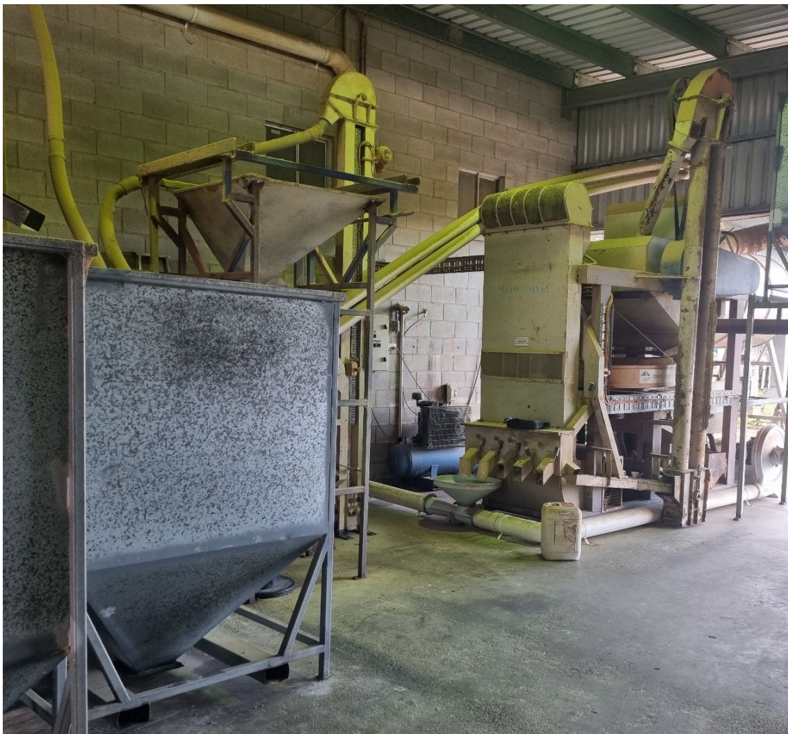
Figure 16.10: Typically, a dry mill is undercover and has a receival station, a huller to remove the parchment and a polisher to remove remaining parchment, which is then size-graded through a series of sieves before passing over a densimetric table to sort out defective beans.
