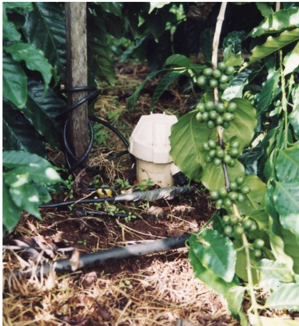
Figure 10.2: Moisture probes can be set for full point and refill point from a range of soil depths to assist in irrigation scheduling.
