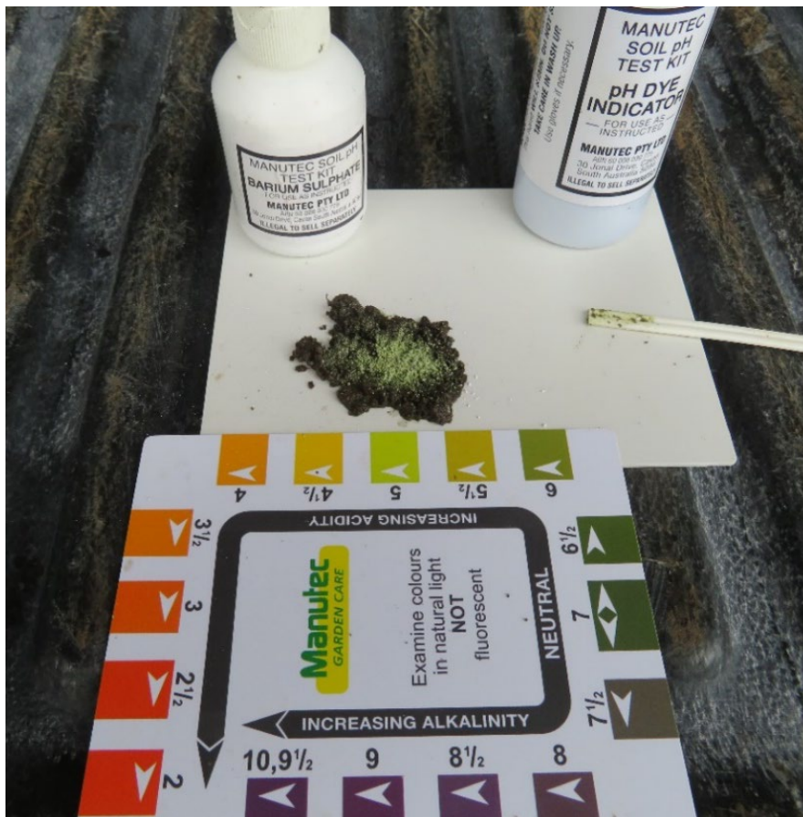
Figure 9.21: A quick, easy-to-use test for pH in the soil. This sample shows a pH between 5 and 5.5. Ideal pH for coffee is between 5 and 6. These test kits are available from retail outlets.
