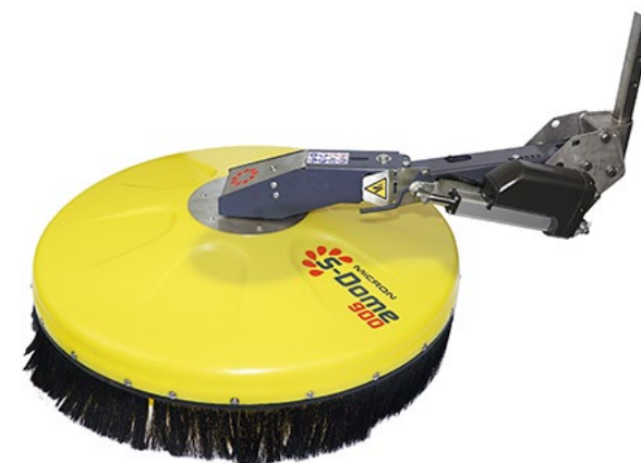
Figure 13.18: A sprayer shielded under a dome minimises the risk of overspray on young coffee trees.
