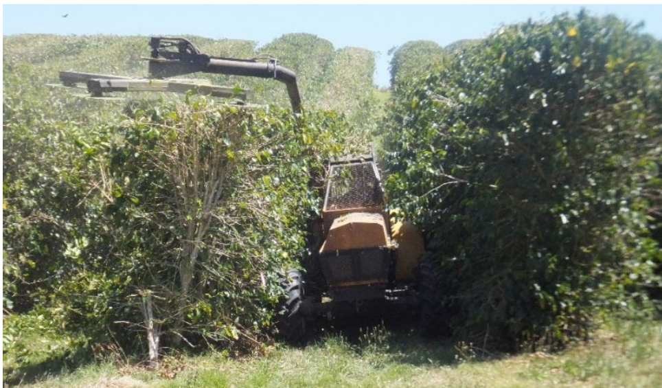
Figure 14.5: A multi-purpose hedger, with circular saw blades on a rotating arm, can be used to prune the tops and sides of taller varieties.
