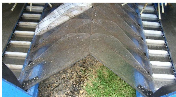
Figure 15.13: Harvesting low-hanging branches is achieved with the use of crop lifters in the front of the machine.
