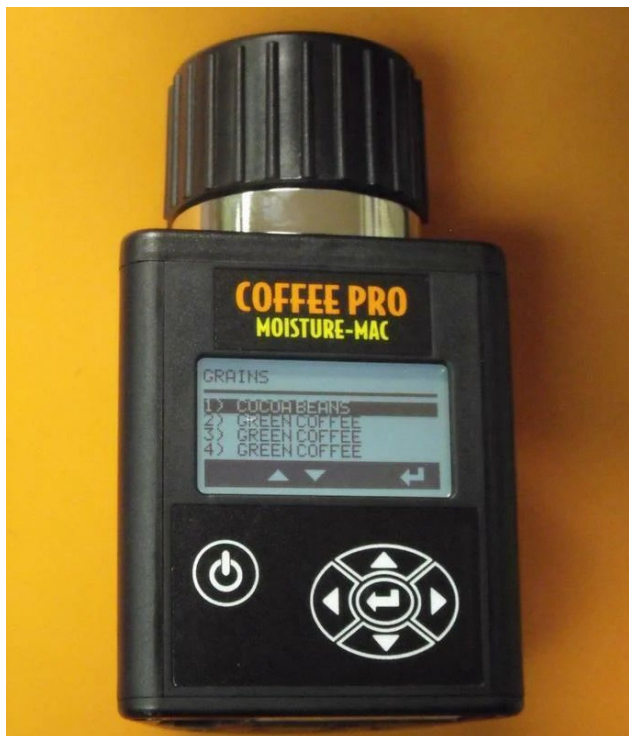
Figure 7.1: The moisture content of coffee seed is tested using a grain moisture meter. When storing seed for propagation, a moisture content of 40% will ensure maximum viability. This is a helpful tool in the nursery and the processing shed.
