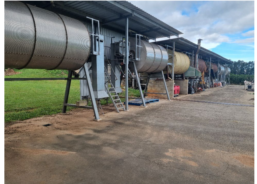
Figure 16.7: Horizontal rotary driers can dry parchment or naturals.
