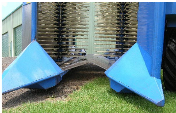
Figure 15.13: Harvesting low-hanging branches is achieved with the use of crop lifters in the front of the machine.
