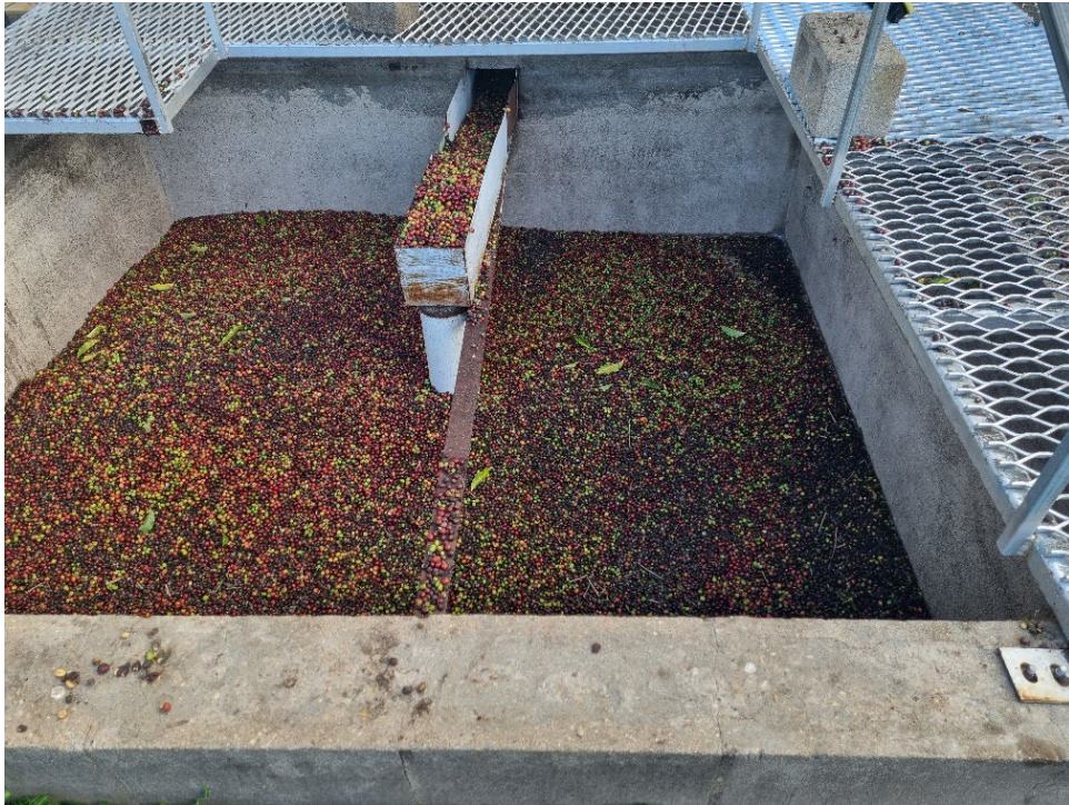
Figure 16.3: Receival – the harvester dumps the cherry crop directly into the receival tank prior to pulping.
