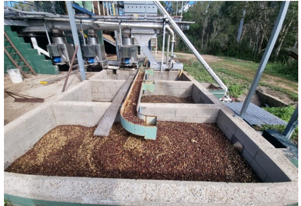
Figure 16.4: Large processing plant with three in-line stainless steel pulpers in the background. Waste pulp collecting in tank.
