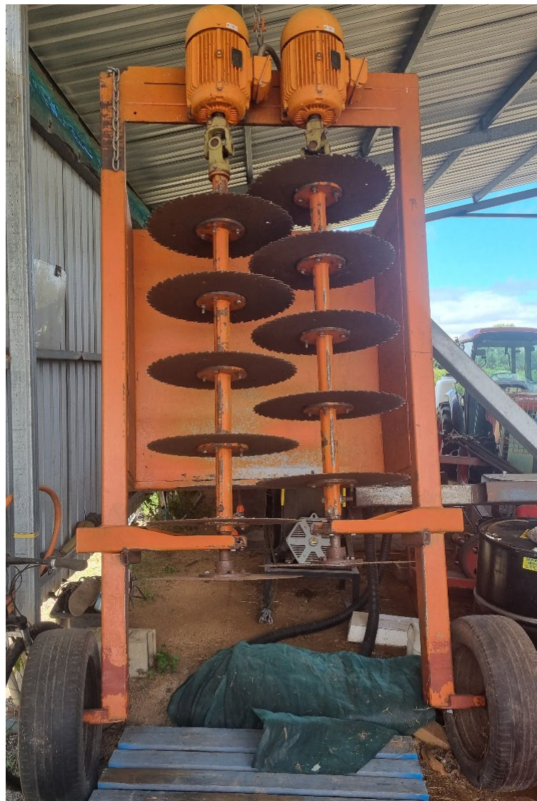
Figure 14.7: This tree shredder is used to shred trees to knee height. Remaining side shoots are also cut off, leaving a stump that will regenerate and bear a crop after two years. The prunings are shredded into pieces less than 30 cm, which readily break down and do not interfere with any cultural operations. Best done a block at a time every 6–8 years.
