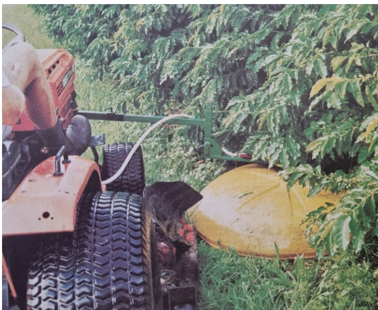
Figure 8.10: A dome sprayer head with a low drift nozzle will minimise herbicide contact and damage to the seedlings.
