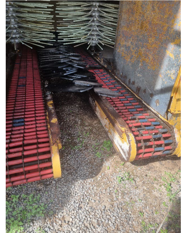
Figure 15.11: The flat leaf and twig extraction rollers at the rear of the machine allow efficient removal of waste and prevent costly blockages and damage to the machine.
