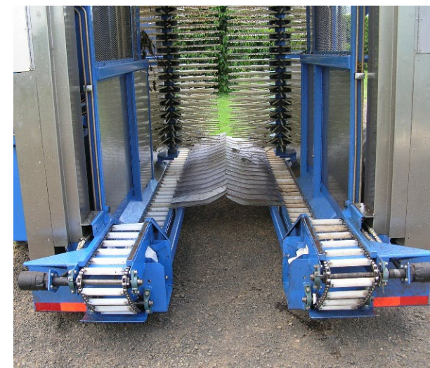
Figure 15.15: This rear view of the harvester shows how harvested cherry is conveyed through the harvesting bin on the side of the machine. Leaves and twigs are blown out of the rear of the machine.
