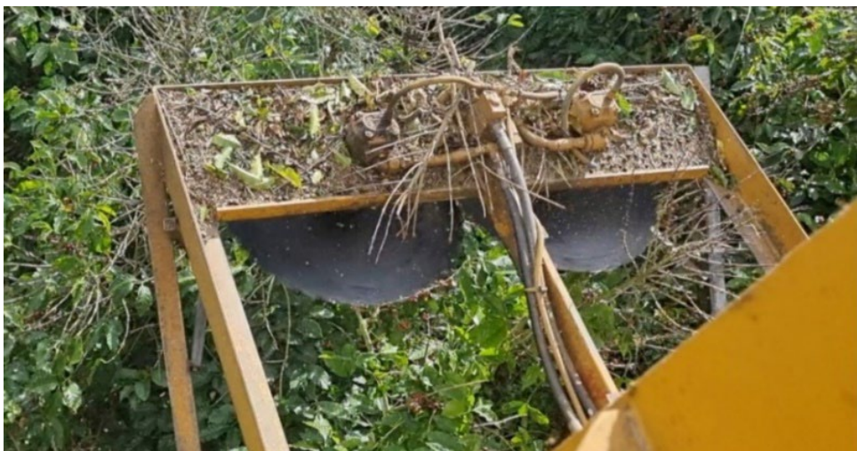
Figure 14.6: A pair of circular blades mounted at the top and back of the harvester is used to 'cap' the trees after the last pass each harvest season. This maintains trees at optimal harvestable height.
