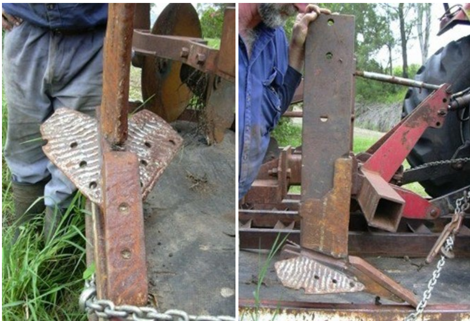
Figure 6.4: The 'winged keel' implement uplifts the soil, shattering compacted layers without disturbing the soil surface.
