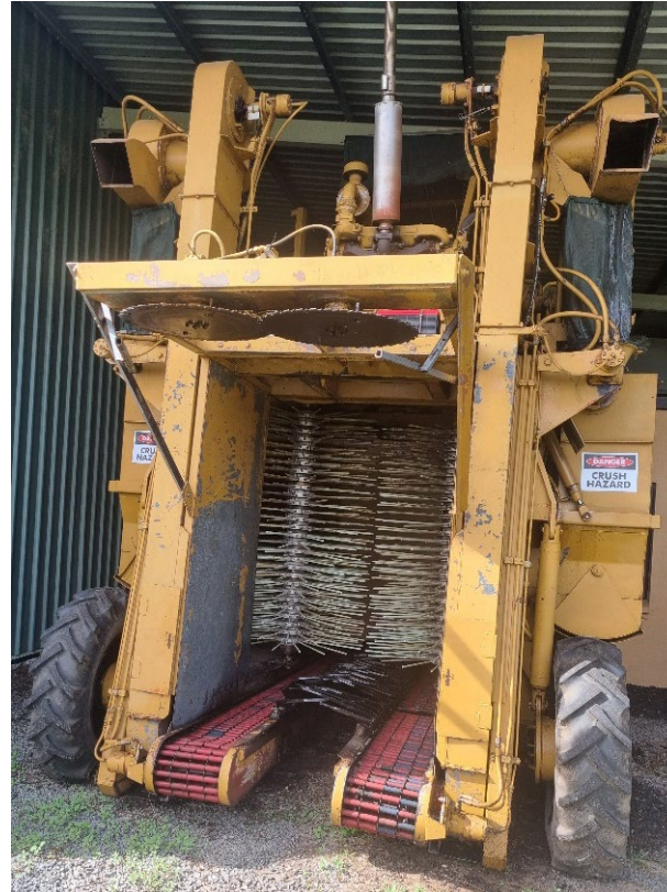
Figure 15.11: The flat leaf and twig extraction rollers at the rear of the machine allow efficient removal of waste and prevent costly blockages and damage to the machine.
